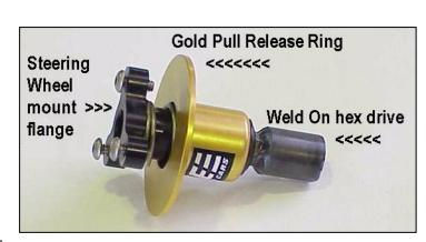
and the KLRC steering wheel bolts to the three bolt mounting flange. Pull the gold ring flange back and the
