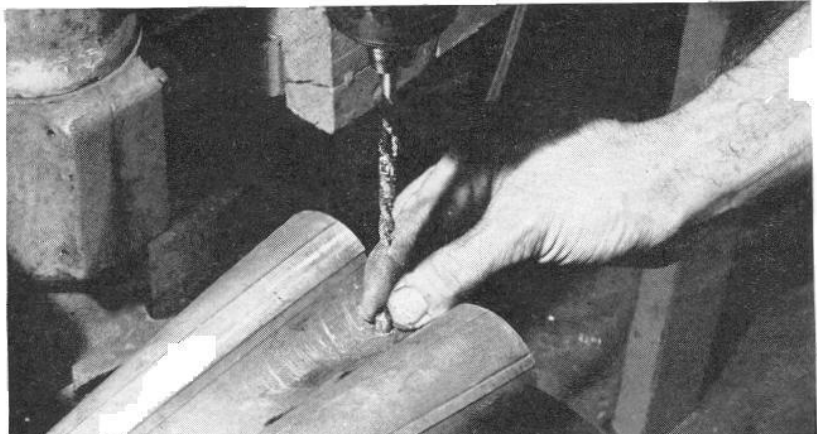
A stock retaining pin, 7/8" from the rotor end, is backed up another pin in a different channel. A 1/4" hole is drilled, then reamed with a taper reamer until the pin will drop into the hole, allowing the head to protrude only 1/16 inch.
