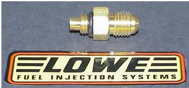
**Nozzle Holders** – we use and recommend brass for nozzle holders even if they are a little more expensive they are significantly more robust as we find the aluminium nozzle holders tend to split where the nozzle screws in. If you want aluminium nozzle holders we can provide them as well. Aspirated nozzle holders are used in normally aspirated and non boosted applications above the blower. Non aspirated are used below the blower and after the turbocharger.
