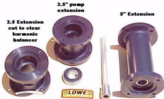
Extension assemblies include bearing and driveshaft
