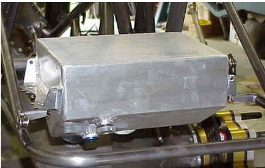
Puke tank on the back of an altered with sight gauge.
